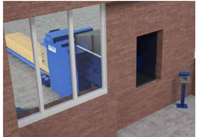
Filling in wall connected hopper
