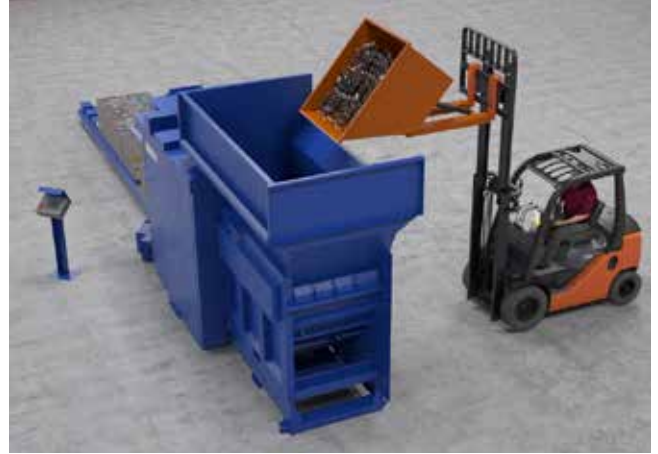
Filling by means of a lift truck
