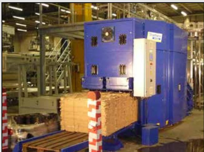
According to Mr. Carsten, head of the Gerolsteiner facility management department, the last old horizontal baling press used for the compression of perforated PET bottles, is now to be replaced by a Strautmann briquetting press.
